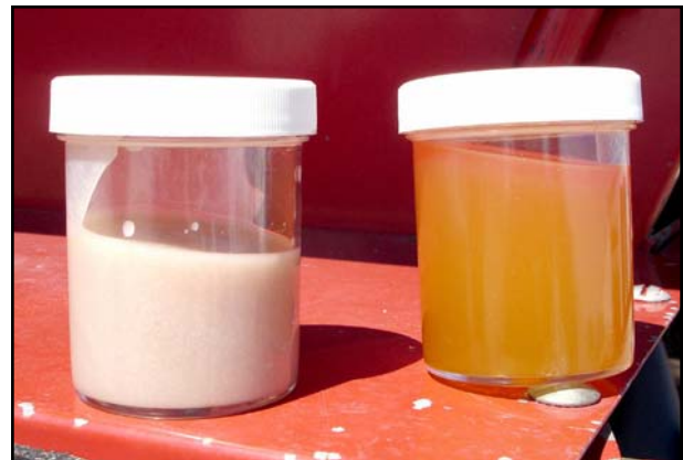
These fuel samples were retrieved from a tractor damaged by animal fat biodiesel. The sample on the left was found within the fuel system and the other was taken from the fuel filter.
